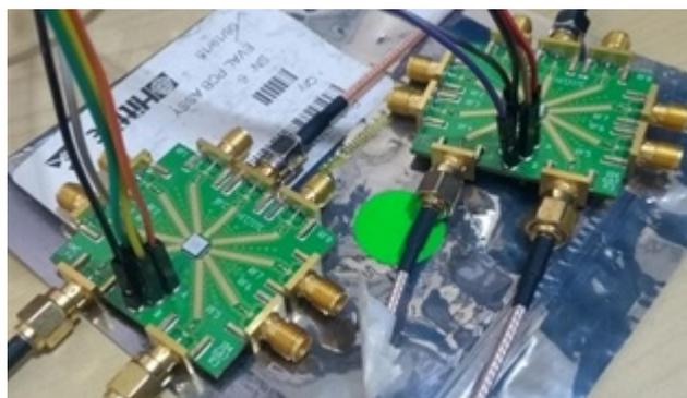
Figura 26 – Switches HMC253ALC4 (ANALOGDEVICES, 2018).
